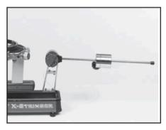
When the correct tension is attained, the drop weight bar will rest horizontally as shown. For accurate tensioning, it must be lowered and come to rest at horizontal without assistance. Manually forcing the tension bar to the horizontal position will greatly increase the string tension and may result in racquet damage.
